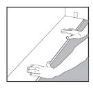
Turn the tongue side of the plank facing the wall. Maintain a gap of a 5mm on the short side.
